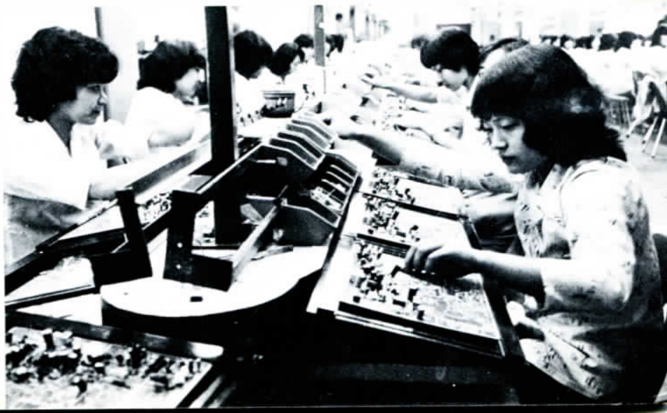
At the Luks Electronic Co., Ltd., a factory built solely with funds from Hongkong produces connection plates for 14-inch colour TV sets.
