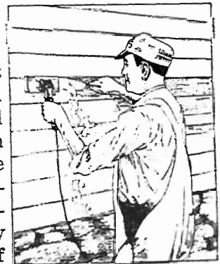
This is an electric paint burning and scraping machine. Result: unemployment for painters.
